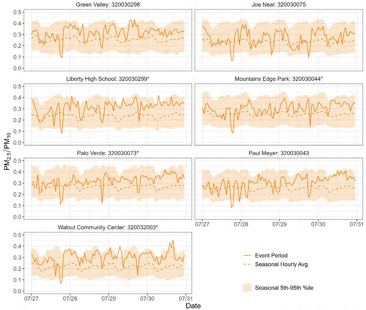
Figure 172. Ratio of PM_{2.5}/PM_{10} concentrations recorded at the Green Valley, Joe Neal, Liberty High School, Mountains Edge Park, Palo Verde, Paul Meyer, and Walnut Community Center sites during the July 28-29, 2022, event period. The 5-yr average PM_{2.5}/PM_{10} diurnal ratio is displayed as a dotted line, and the 5th-95th percentile range is shown as a shaded ribbon. The 5th-95th percentile concentration is calculated across the ozone production season (May-October) of 2018-2022.
